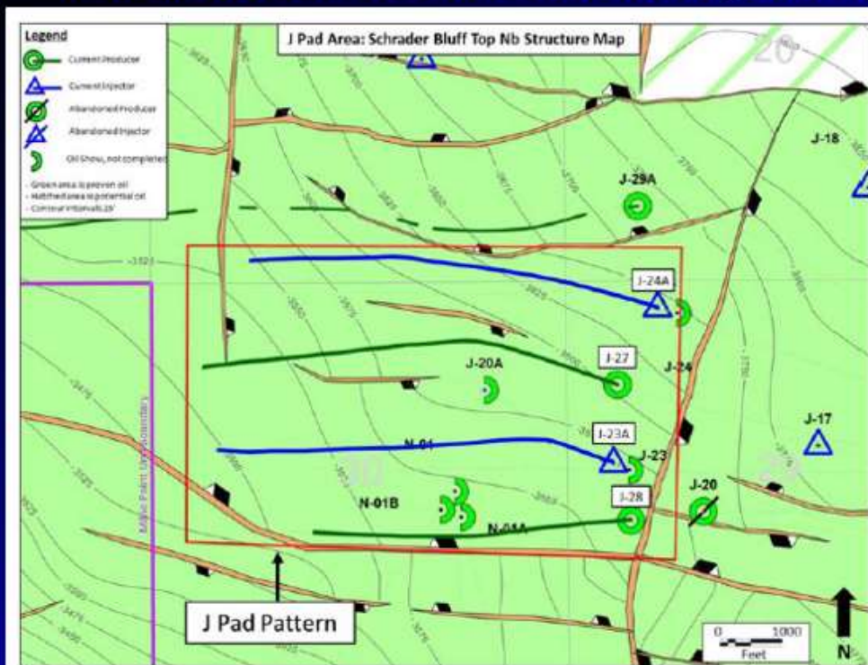
Figure 11—Location Map of J Pattern, well inside red box part of initial pattern and wells outside were drilled as part of expansion
